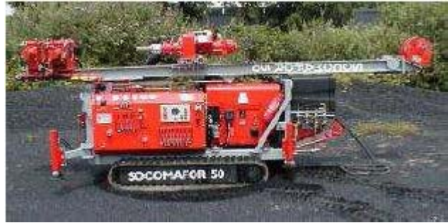
Figure 2 : machine de forage, flèche horizontale
